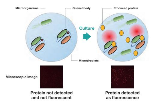
The diagram shows droplet screening theory (case of protein production bacteria). The produced protein emits fluorescence when combined with Quenchbody. By selecting droplets with high fluorescence, strains with improved protein secretion can be obtained.
